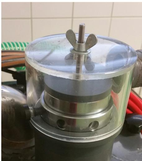
FIG 1: Expiratory flow regulator with semi-closed orifices.
