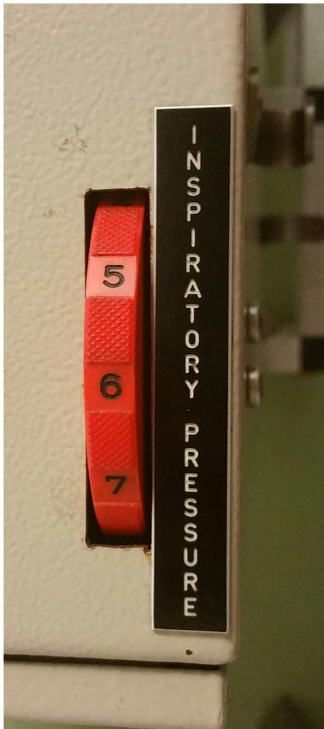
**FIG 4:** Peak inspiratory pressure-limiting device.
