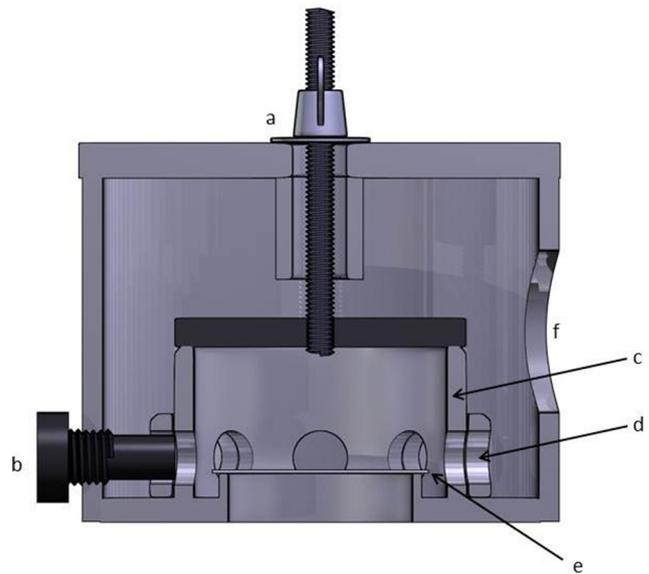
FIG 2: Diagram depicting a transversal cut section of the expiratory valve of the Smith L.A.-90 ventilator. (a) Acrylic cup holding screw (b) Plastic screw fixating the steel rings with orifices, (c) Inner ring of the steel rings with orifices, (d) Outer ring of the steel rings with orifices, (e) Unidirectional valve disc (not depicted in figure 3 to facilitate visualisation of gas flow), (f): Connection to active gas scavenging system
